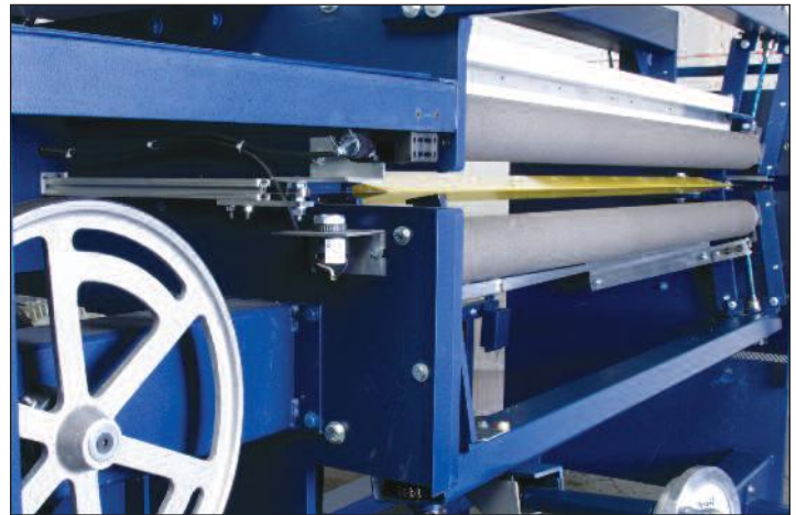
Adjustable pinch roller, heavy-duty blade guide, and blade
